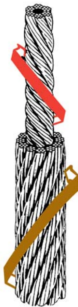
Example of a 2-layer rotation resistant construction with 12 outer strands. (19x7)
